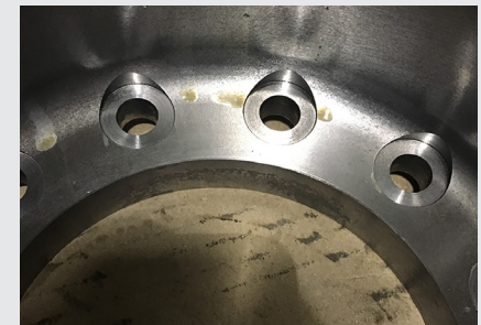
After: Spotfaces made with the HEULE BSF.
