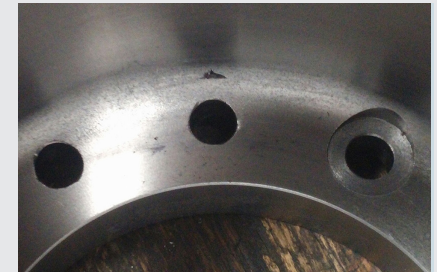
Before: Tool failure after one hole due to interruption.
